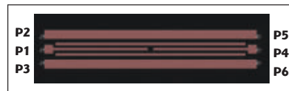
▲ Fig. 1 Schematic of the CPW Ka-band bandpass filter.
